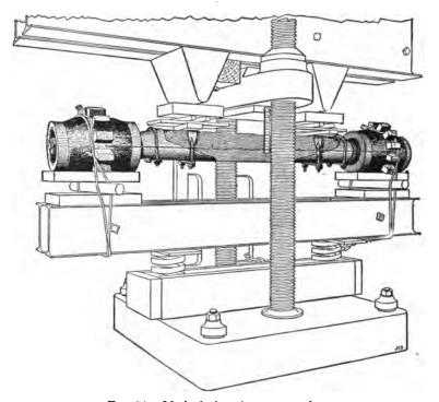
Fig. 54.—Method of testing wagon axles.
